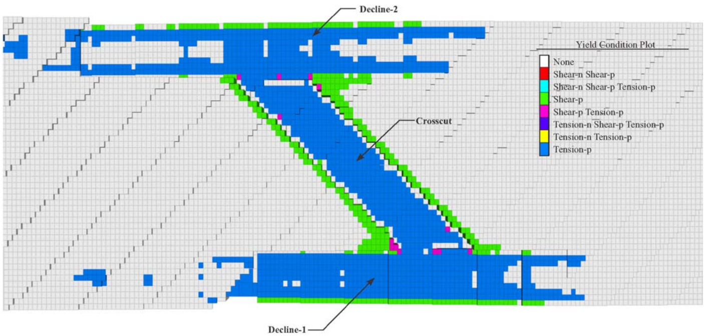
Fig. 8a. Yield condition plot in inter-decline crosscut, arched-support scenario (plane parallel to crosscut floor).
