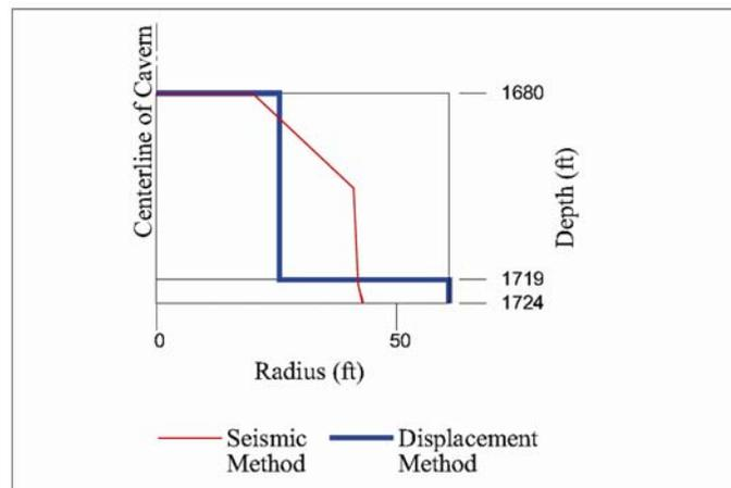
**Figure 8. Comparison of Top of Cavern Shape from the Seismic and Displacement Methods**
