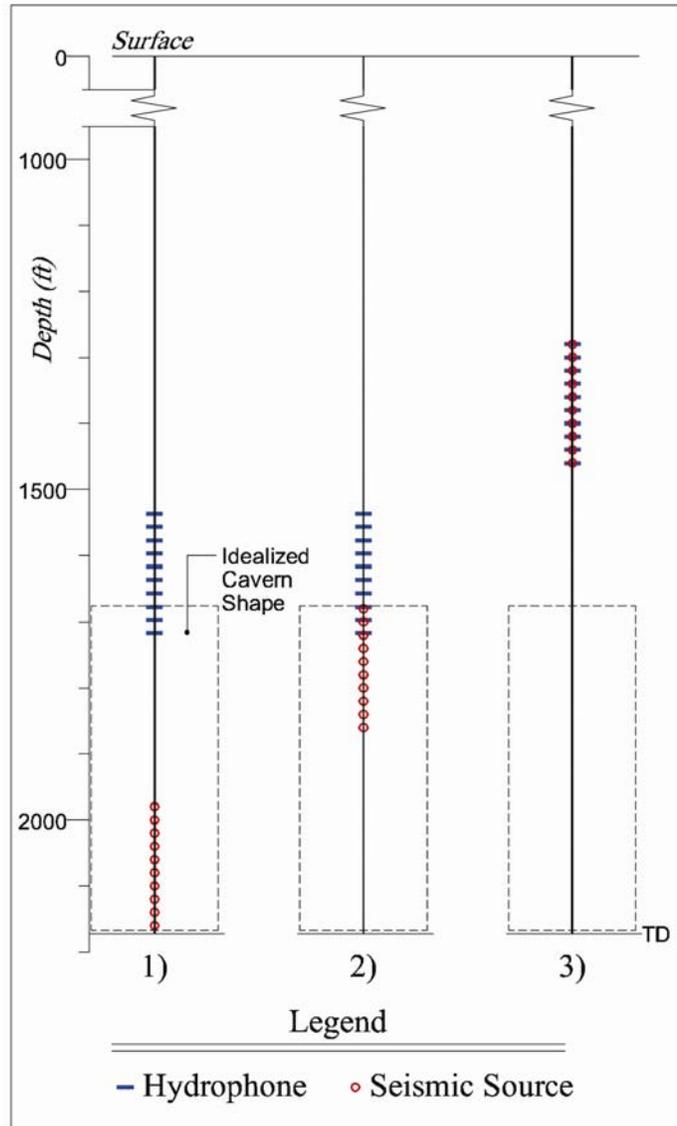
Figure 2. Positions of Hydrophones and Sources
