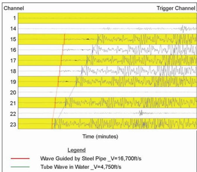
Figure 4. Example Seismic Record
