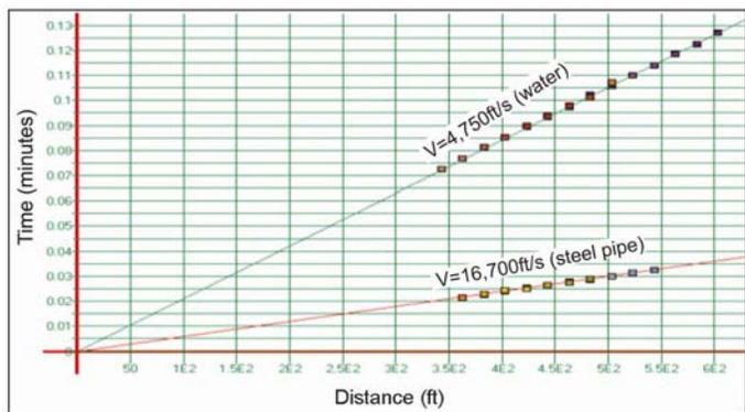
Figure 3. Seismic Energy Velocities
