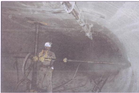
Figure 4. Agapito Associates, Inc. Overcoring CP-65 Drill Setup in a Trona Mine
