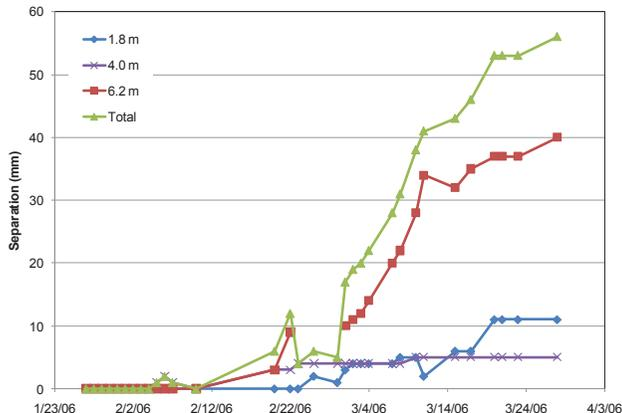
**Figure 6. Plot of roof movement for station 9 – Copper Mine.**
