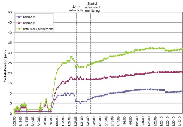
**Figure 12. Roof movement for station H MCC.**
