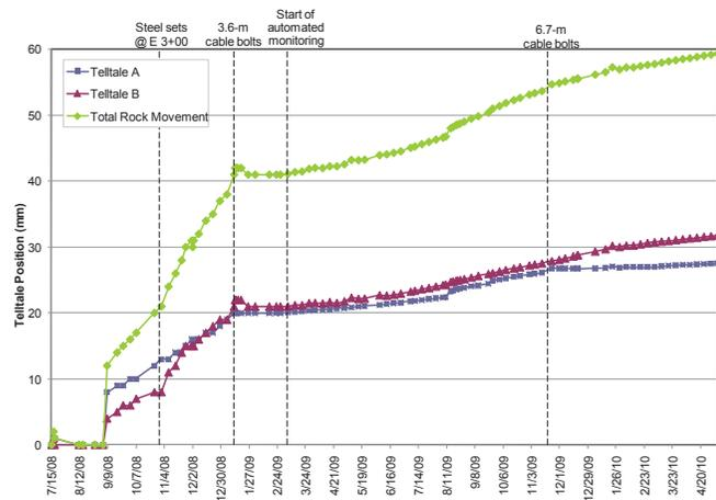
**Figure 11. Roof movement for station E 2+50.**
