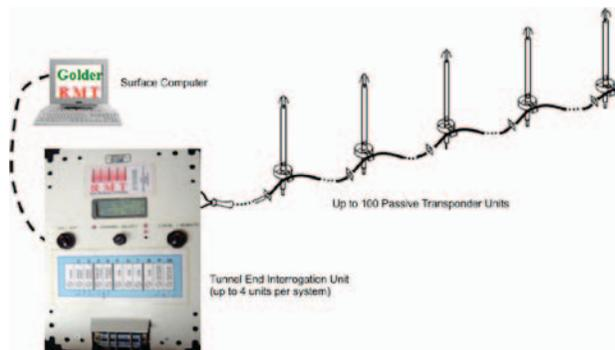
**Figure 2. Automated telltale network installation.**
