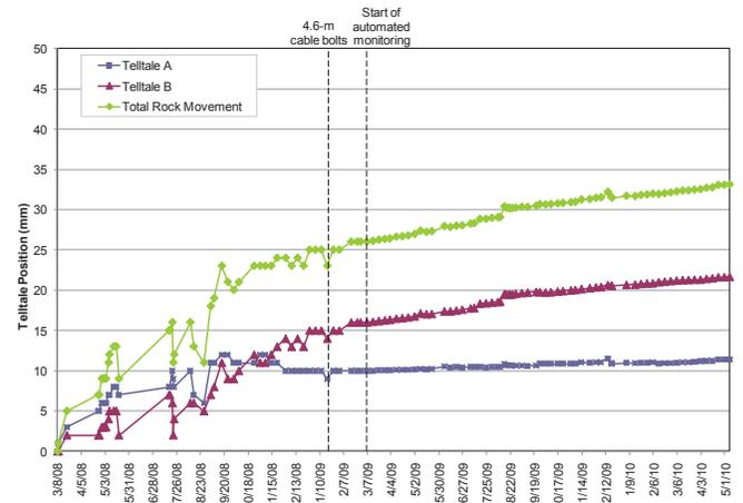
**Figure 9. Roof movement for station A MCC.**
