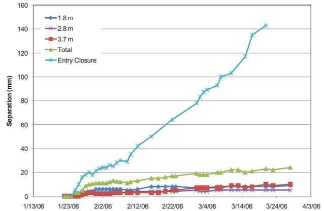
**Figure 7. Combined roof movement and entry closure for station 3.**
