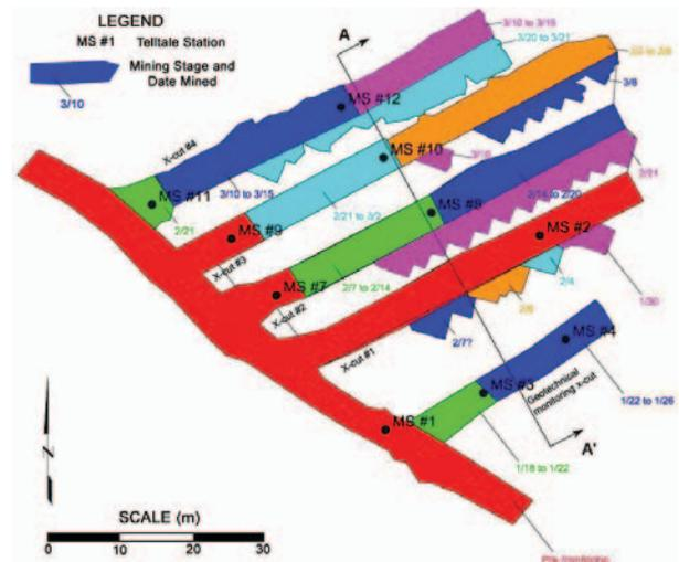
Figure 3. Mine layout and telltale locations – Copper Mine.
