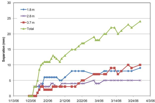
**Figure 5. Plot of roof movement for station 3 – Copper Mine.**
