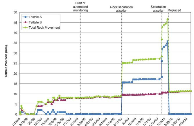
**Figure 10. Roof movement for station E 1+00.**
