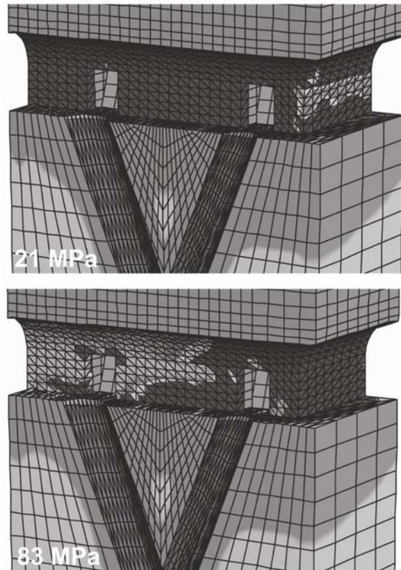
Figure 10: Comparison of Liner Damage in the Draw Lines using Normal (21 MPa) and very High (83 MPa) Strength Concrete in Weak Andesite
