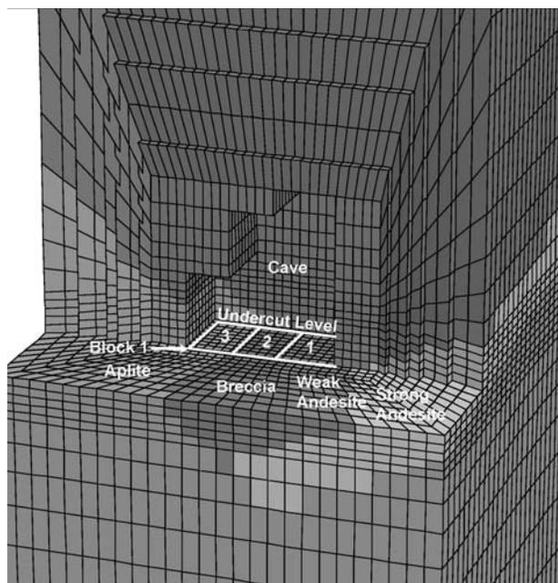
Figure 5: Block 1—D Orebody Abutment Stress Model Geometry and Rock Types
