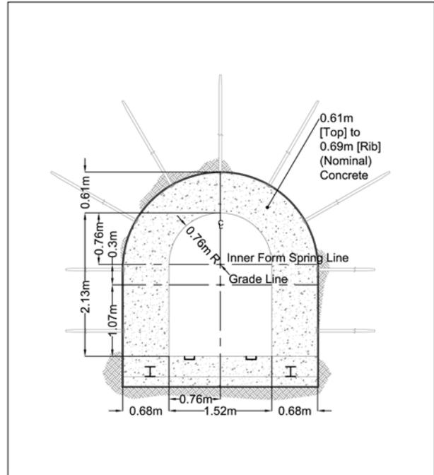
Figure 7: Proposed Support Design for the Grizzly Level Draw Lines
