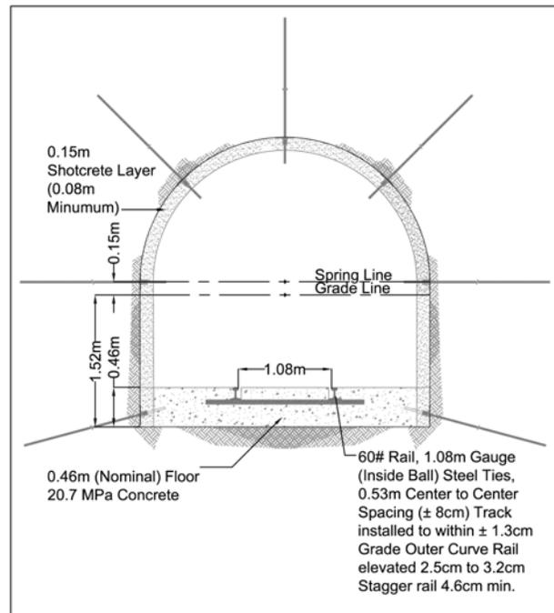
Figure 8: Proposed Support Design for the Haulage Level Drifts
