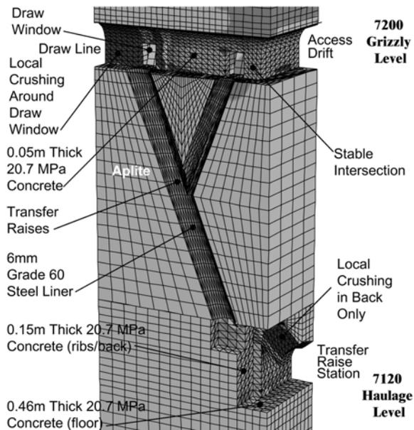
Figure 9: Transfer Raise System Model and Liner Yielding during Abutment Loading in Aplite
