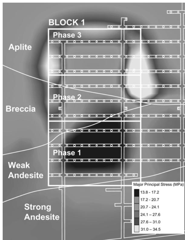
Figure 6: Peak Abutment Stress Map at the Final Stage of Undercutting—Grizzly Level, Block 1
