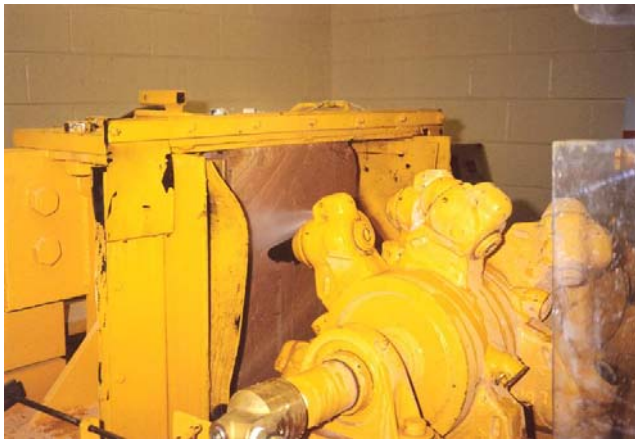
Figure 2. 1 The automatic rock & coal rotary cutting simulator
